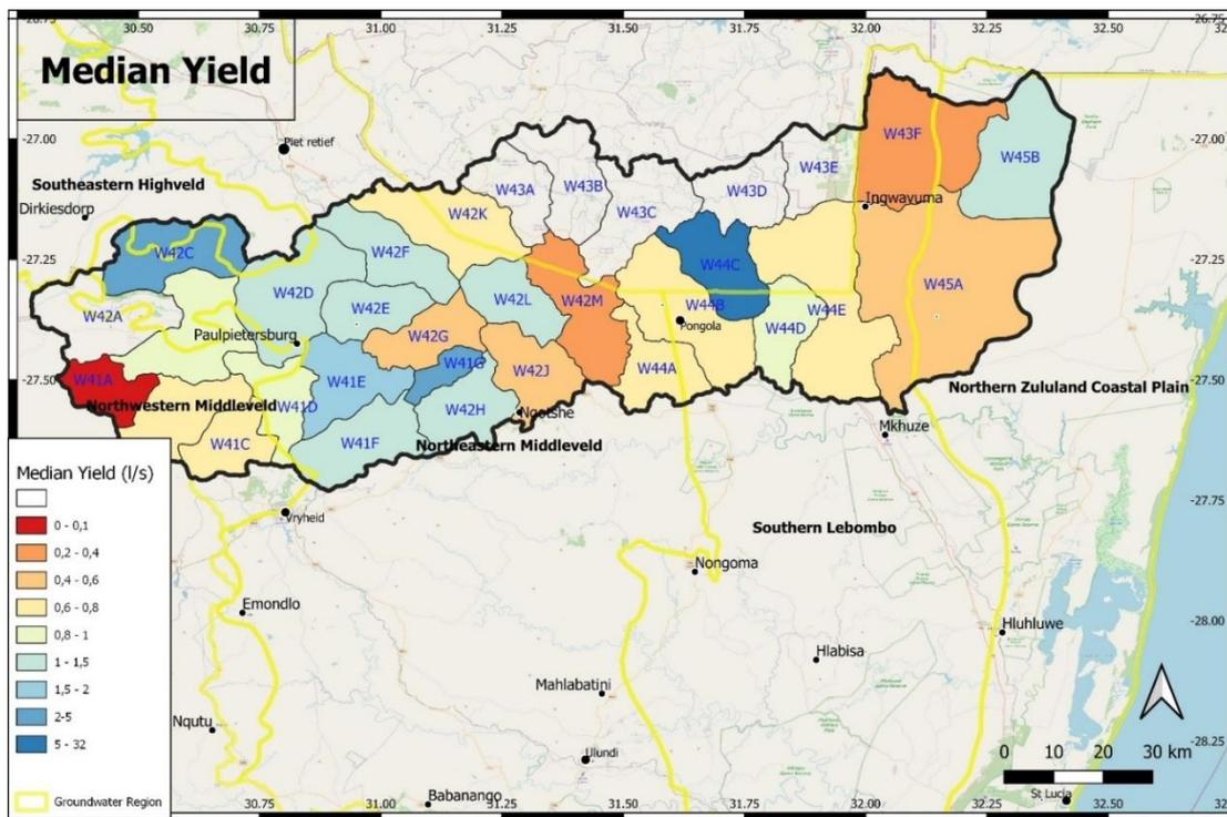
**Figure 3.8 W4 Catchment: Median borehole yields**
